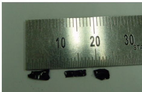
Fig. 3. CNF/Ppy composite samples fabricated by an SH process.
